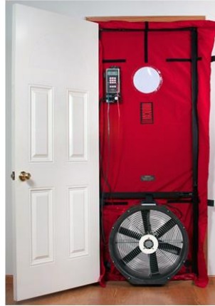
Figure 4: Air tightness test
