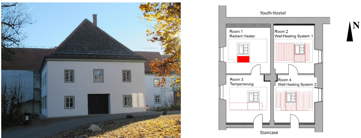
Figure 1. Left: The “Alte Schöfflerei” (old cooperage) at Benediktbeuern Monastery, after façade restoration in 2015. The measurement rooms are on the ground floor in the left building part (behind the scaffolding), the so called Northern-Building. Right: Ground plan with different examined wall heating systems in the four measurement rooms.
