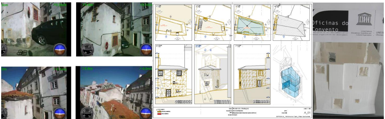
Figure 2. Drone flight images (left), Autodesk Revit 2012 model exported to dynamic simulation software as Ecotect and OpenStudio/EnergyPlus using gbXML (middle) and 3D printed model (right) (source: author).
