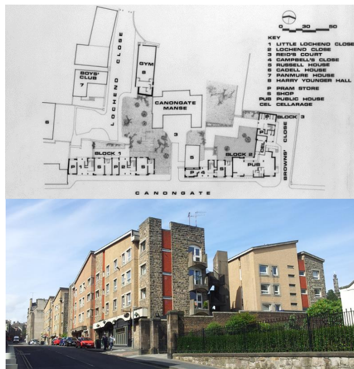
Figure 1. Ground floor plan of the Canongate Housing complex and photograph along Canongate with blocks 2 and 3 in the foreground (Image © left: HES (Spence, Glover and Ferguson Collection) Licensor canmore.org.uk; right: HES)
