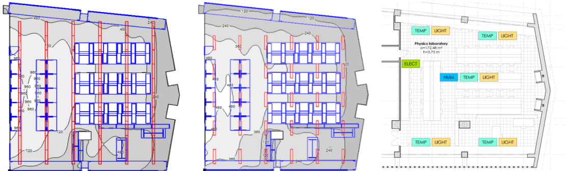
Figure 2. Lighting simulation results with all lights on (left) or half of the lights on (centre); deployment of monitoring network in the physics laboratory (right)
