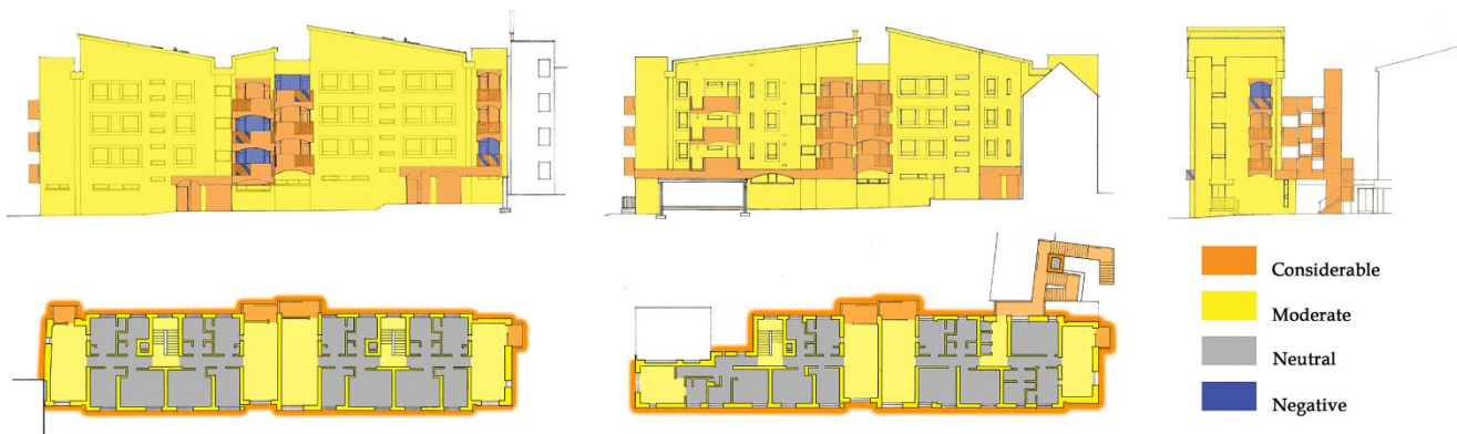
Figure 2. Example of colour-coded drawings in the conservation statement, illustrating the significance levels of different building elements and spaces of blocks 1 (left) and 2 (right) (Image © Simpson & Brown Architects)
