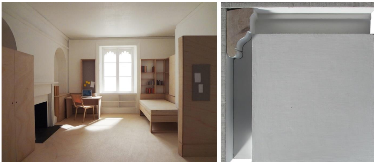
Figure 4. Photograph of 1:10 scale model and of full-size maquette of cornice detail, exploring the form of the insulated lining and joinery and the relationship of the insulated lining and historic cornice.
